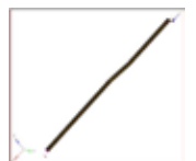
Figure 12 FE model of the drag link
